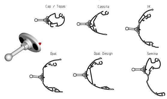
When the awning opens, the ball-shaped heads retract into the retainer on the stationary wind support. The wind support needs to be set to the height of the drop profile.
