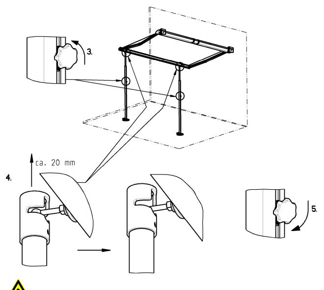
Do not lock in the wind support by turning the rotating head!
