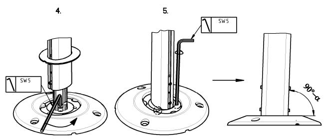
Once the required angle is reached, re-tighten the screw located in the centre of the adjustment base (4.) and re-tighten the four grub screws at the bottom end of the wind support (1.)
